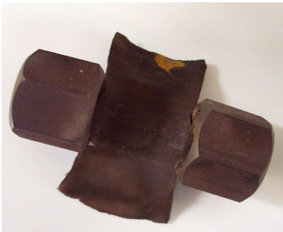
Fig. 7. Fragments of the testing set-up of the small-scale cook-off test after DNPT testing.
