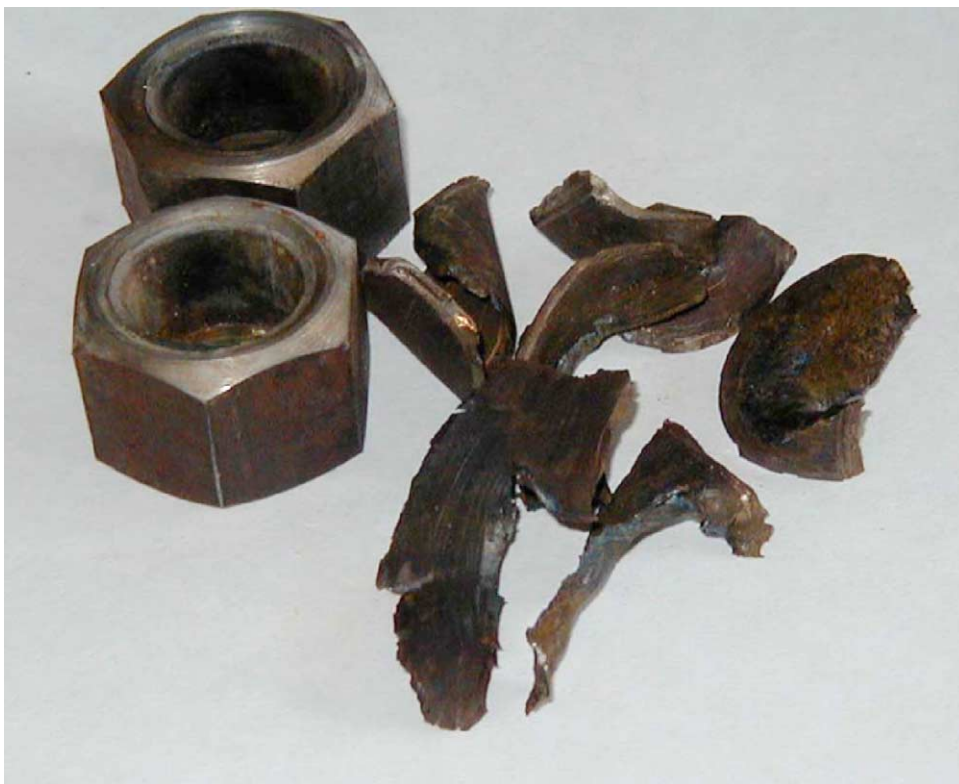
Fig. 6. Fragments of the testing set-up of the small-scale cook-off test after DPT testing.
