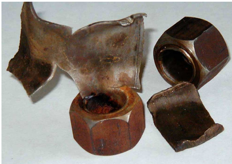
Fig. 8. Fragments of the testing set-up of the small-scale cook-off test after HEXADI testing.
